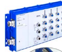
OCTOPUS OS32-0816020606TPEP (942 069-003) managed ruggedized IP54-Switch 18 Ports including 8 ports PoE, M12 „D“ coding, 8 ports 10/100 Mbit/s, M12 „D“ coding 2 ports 1000BASE-SFP sockets Approvals: CE, C-Tick, GOST-R, EN 50155
